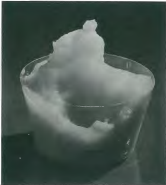
FIG. 2. The viscous gel appearance of MFC at 3% in water.
